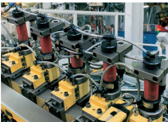
Stamping units placed in line
