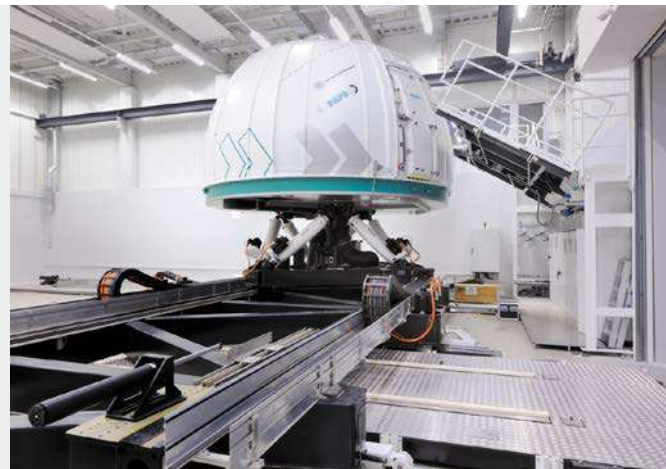
ACE safety shock absorbers protect end positions in two axes of a driving simulator
